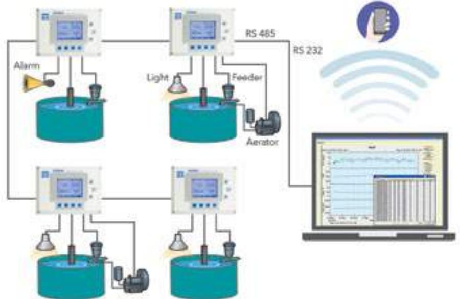
There are many possibilities for connecting the monitors. This is one example of four monitors individually monitoring and controlling four tanks with direct PC connection. E-mail and SMS alarming is available from network-connected PC running AquaManager.
