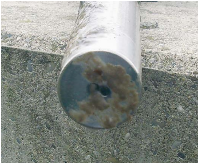
Without ultrasound cleaning system
