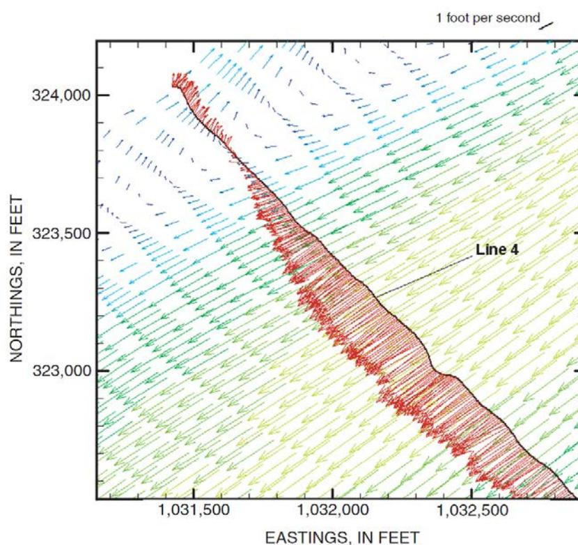
**Figure 1--Measured and simulated 2-D velocity vectors (red arrows are measured by ADCP, multi-colored arrows are simulated by 2-D model). Image from Wagner (2003).**
