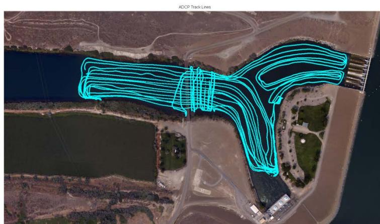
**Figure 2--Aerial orthophoto of study reach showing location of ADCP tracks.**
