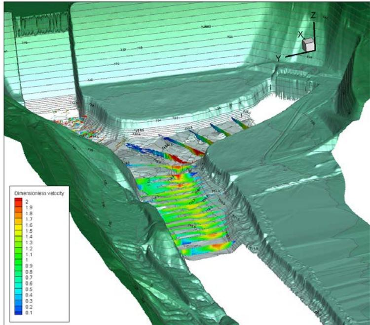
Figure 3--Downstream velocity measured throughout reach.
