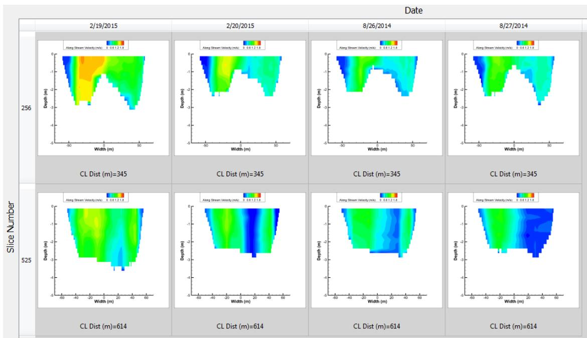
Figure 4--Graph showing downstream velocity from two potential measurement sections for four flow conditions
