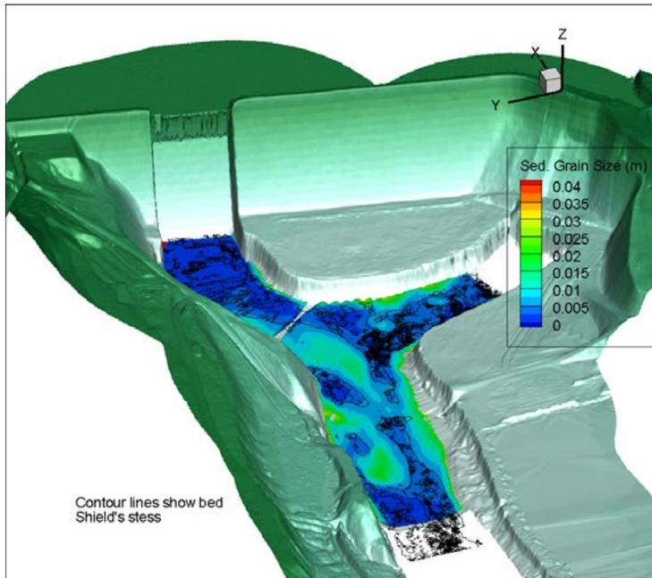
Figure 5--Shield's stress and bed-material size.
