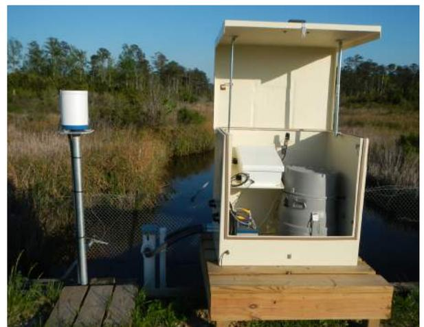
*YSI Systems Stormwater monitoring enclosure with solar power, automated water sampler, cellular based real-time data/event notification, Waterlog rain gauge, EXO water quality instrument and a SonTek IQ flow sensor.*
