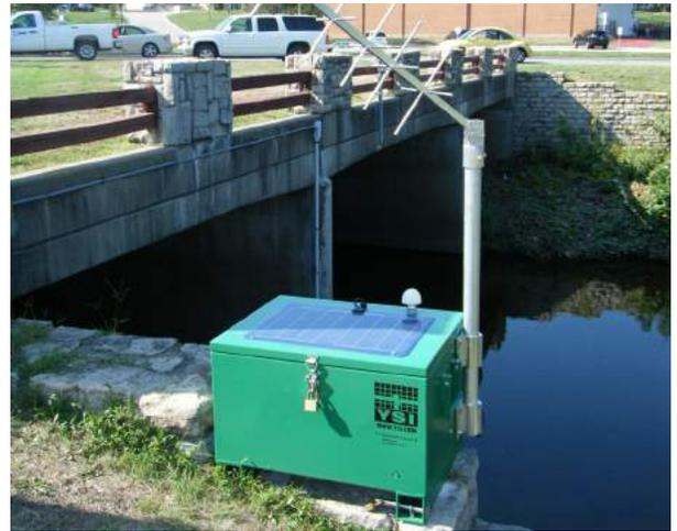
*Portable water quality stormwater site in Kansas equipped with WaterLog GOES satellite data delivery, EXO water quality instrument and solar power.*
