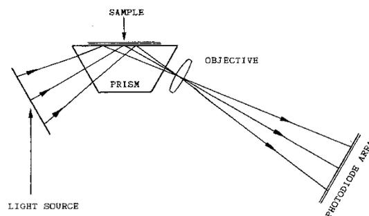
When the composition of a substance changes, so does its RI. Thus a measure of RI can yield information about the composition of a substance. For example, when a substance is dissolved in a liquid the RI increases. Thus a measure of the RI of a sugar solution in water can be used to determine the **solution concentration**.
