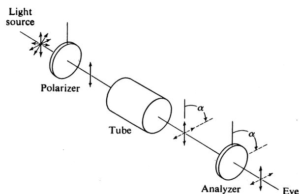
In the sugar industry, the rotation is expressed on a different scale, the International Sugar Scale (ISS), denoted as  $^{\circ}\text{Z}$ . Polarimeters that are designed for particular use in the sugar industry are called Saccharimeter.
