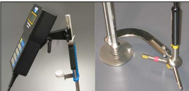
**Figure 1 – SonTek FlowTracker on Top Setting Wading Rod**
