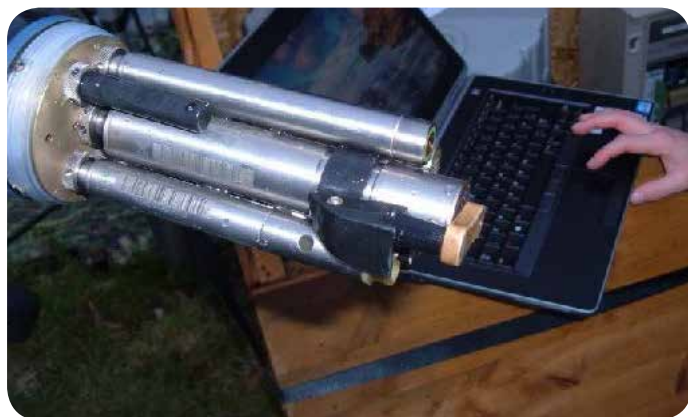
YSI EXO2 sensors (top) and Storm logger cabinet and water sampler (bottom)
