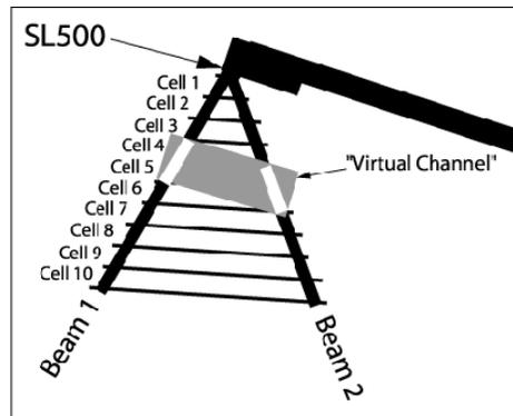
**Figure 7.** Close-up of Fig. 1, showing SL500's range cell locations and "virtual cell" created by the overlap of cells 4-5 on beam 1 and cells 5-6 on beam 2.
