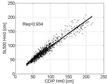
Figure 3. Linear regression comparison between CDIP station 073  $H_{m0}$  and the SL500's internally-computed  $H_{m0}$  showing how well they agree ( $R^2$  0.934). Comparison is for 18 April to 6 June data set.
