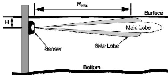
Figure 4. Conceptual diagram of an acoustic Doppler profiler installation, showing the main lobe and a side lobe. The main lobe describes the maximum acoustically-feasible range for the sensor, but the maximum effective range is the intersection of the side lobe with the surface—data beyond this range is likely to be affected. Thus the system's aspect ratio ( $R_{max}/H$ ) is of critical importance for side-looking applications. Modified from Polonichko and Romeo (2007).
