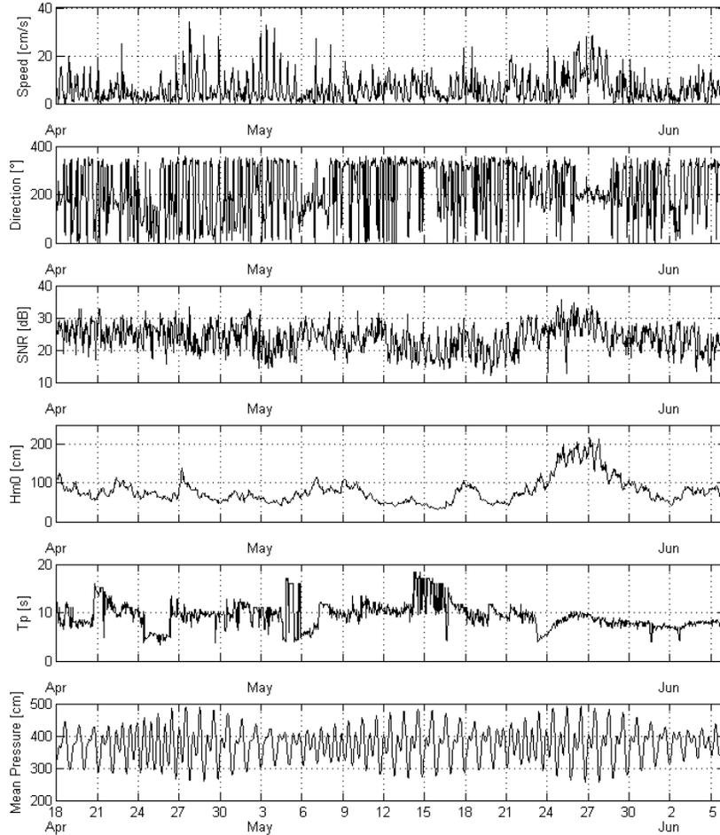
**Figure 2. Time-series of water speed, direction and returned signal strength (signal-to-noise ratio, SNR) data from the 18 April to 6 June data set for the single integrated cell. Significant wave height, peak period and mean water pressure data is also shown for the same time period.**
