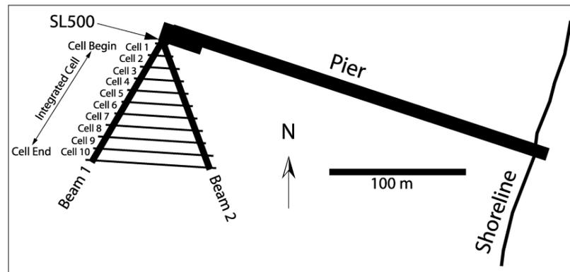
Figure 1. Schematic drawing of Scripps Pier and instrument installation. Both SL500's horizontal acoustic beam paths are shown, drawn to their maximum acoustically-feasible extent. Each individual range cell is shown as well as extent of the single integrated cell. North is 0° direction.
