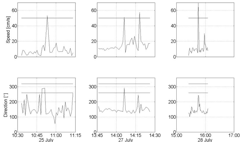
**Figure 8. Computed water speed and direction for 25, 27 and 28 July, processed according to the rip current definition used in this study, inside the “virtual channel”. The horizontal line in the top panels indicates the 50 cm/s threshold used. The horizontal lines in the bottom channel indicate the 260-320° threshold for “offshore” flow direction.**
